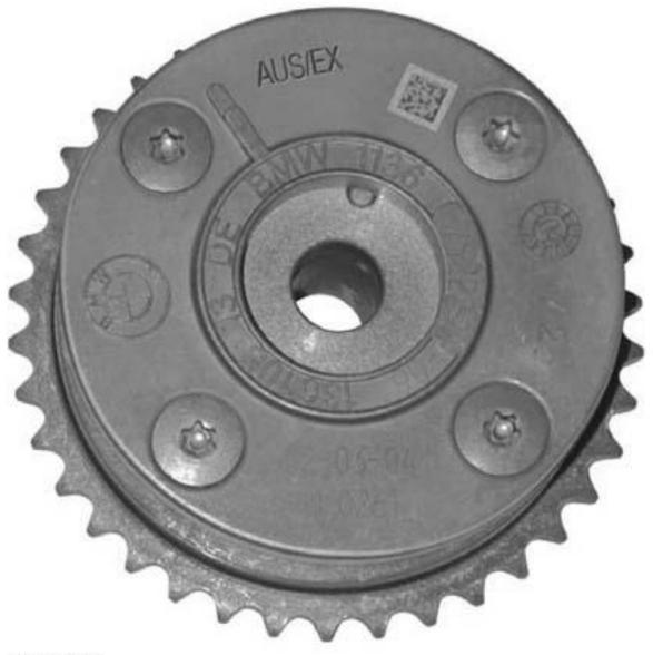
**Fig. 38: Identifying VANOS Unit (Front View)** Courtesy of BMW OF NORTH AMERICA, INC.
