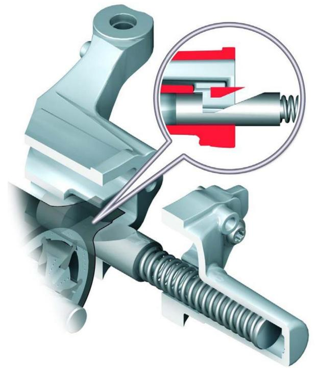
**Fig. 44: Locating Slide Valve** Courtesy of BMW OF NORTH AMERICA, INC.
