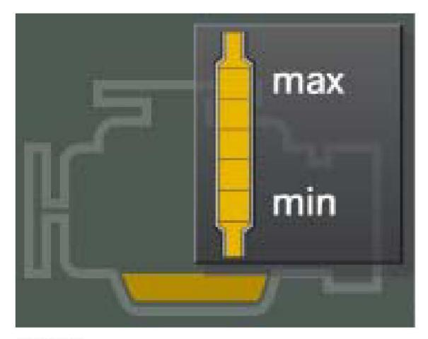
**Fig. 51: Identifying MIL Over Maximum Oil Level Mark** Courtesy of BMW OF NORTH AMERICA, INC.
